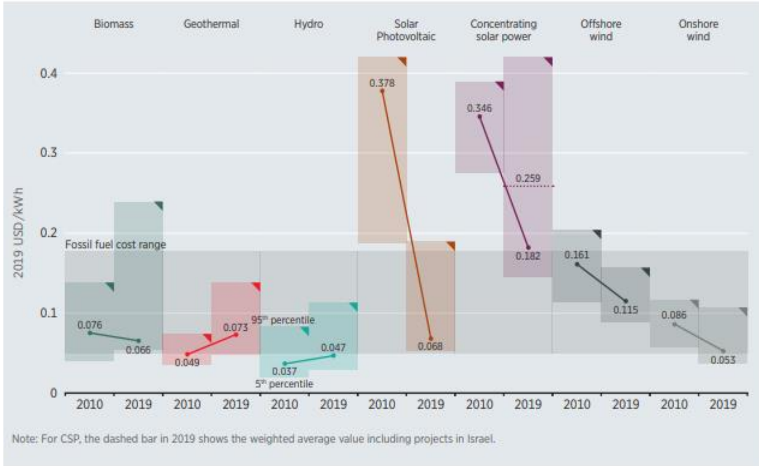
Figure ES.1 Global weighted average levelised cost of electricity from utility-scale renewable power generation technologies, 2010 and 2019
